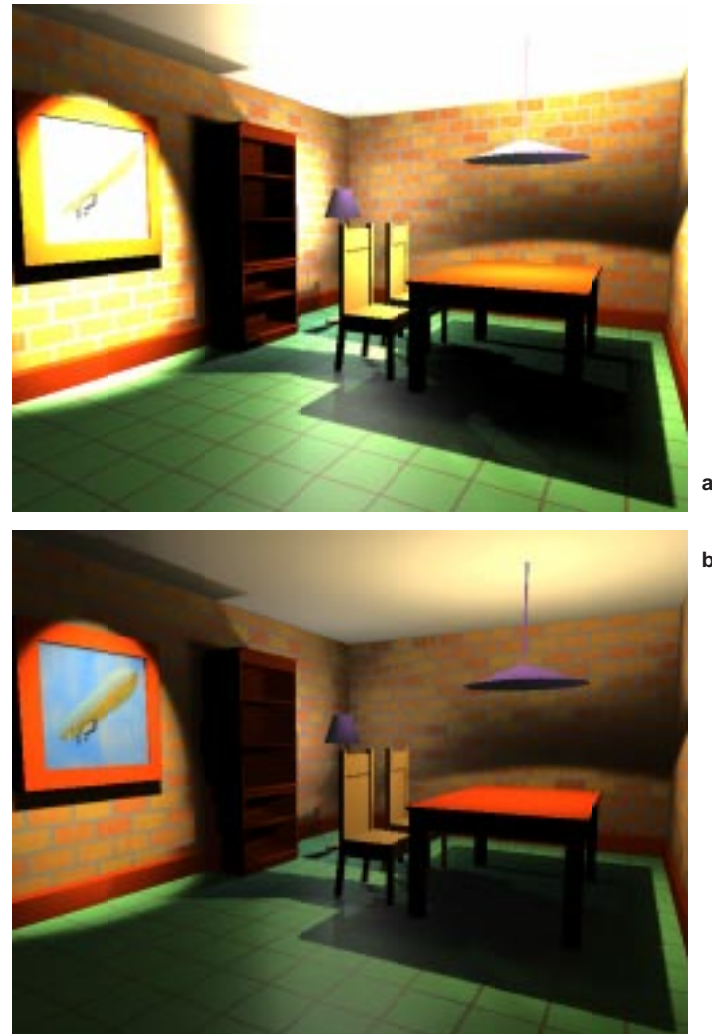
Figure 7.3.2.3: (a) Uncorrected and (b) corrected exposure of a radiosity based rendering.
