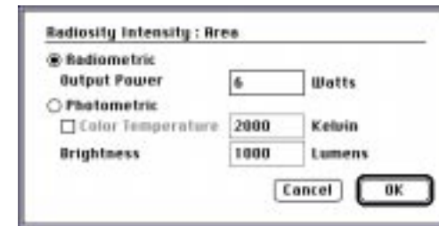
Figure 7.4.4.4: Setting the Radiosity Intensity options for the window area lights.
