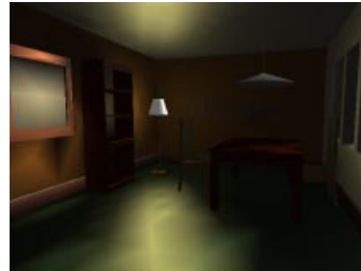
Figure 7.4.3.3: Radiosity rendering of the scene after adding the sun light.
