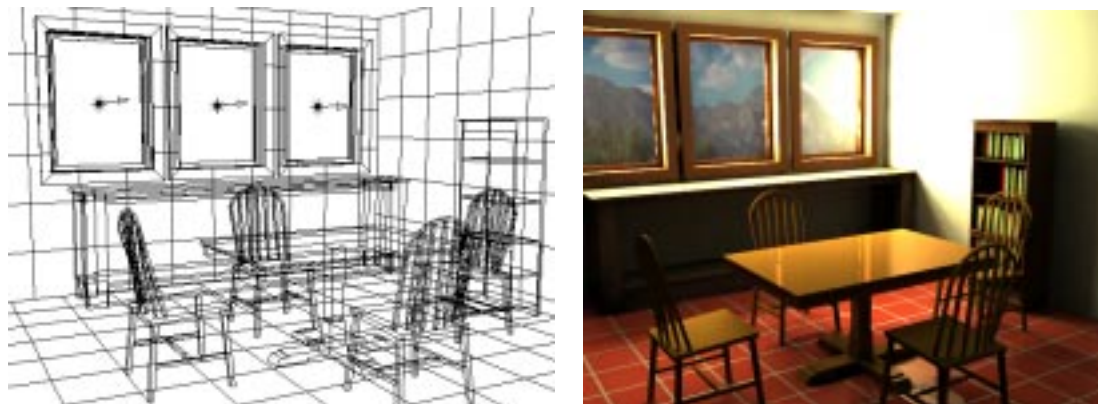
Figure 7.3.1.5: An area light used as an exterior window.
